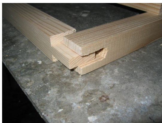
Illustration 2: Ajustement tenon-mortaise
